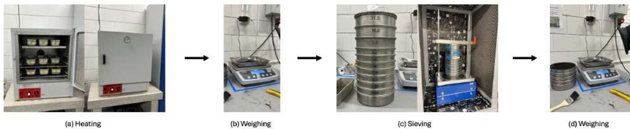
Figure 16. Procedures for sieve test according to the SFS-EN 993-1 standard
