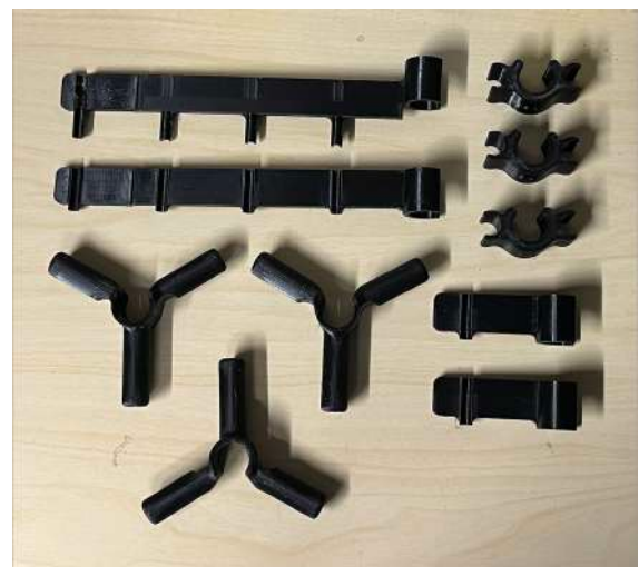
Figure 7A. (a) A part of temperature sensor holder designed on AutoCAD Fusion360 and (b) A set of 3D-printed part
