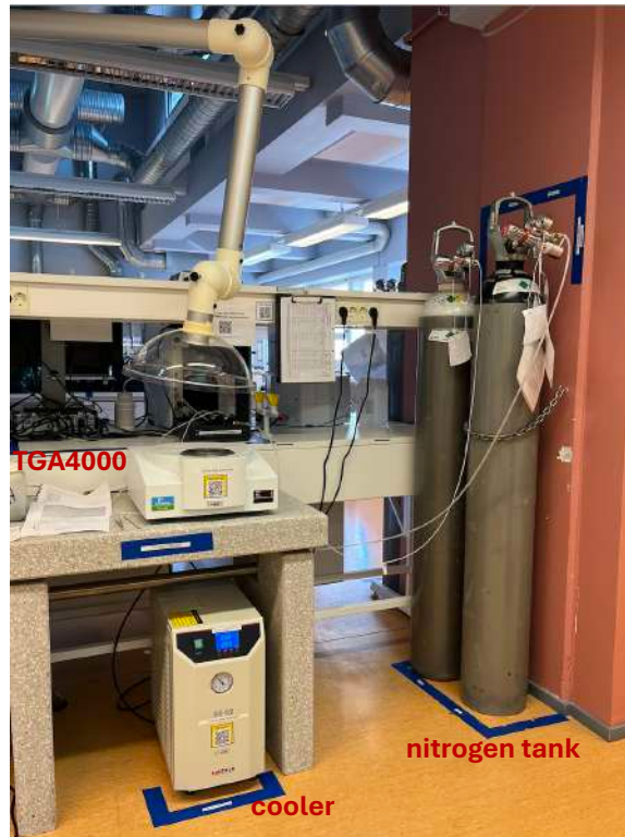
Figure 18. PerkinElmer TGA4000 with nitrogen tank and cooler
